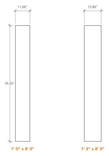
NOTE: BY REQUEST, SIDELITE HEIGHT COMES IN VARYING DIMENSIONS TO A MINIMUM OF 95". EXCESS WILL BE TAKEN FROM BOTTOM RAIL. ALL OTHER DIMENSIONS WILL REMAIN THE SAME.
