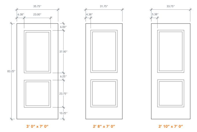
NOTE: BY REQUEST, DOOR HEIGHT COMES IN VARYING DIMENSIONS TO A MINIMUM OF 83". EXCESS WILL BE TAKEN FROM BOTTOM RAIL. ALL OTHER DIMENSIONS WILL REMAIN THE SAME.
